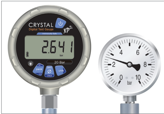
Checking the accuracy of an analog pressure gauge against the display of the Crystal reference gauge
